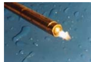
Ignition lance with high energy spark.
